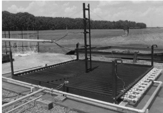
Figure C-3: Vertical rake used to perform simultaneous heat flux measurements at multiple locations.
